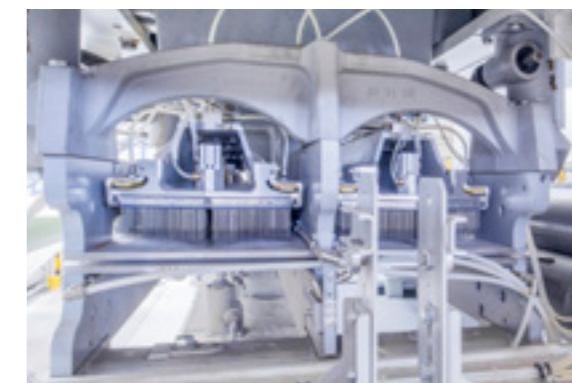
Needlelooms: Pneumatic centralized needleboard pinning system
