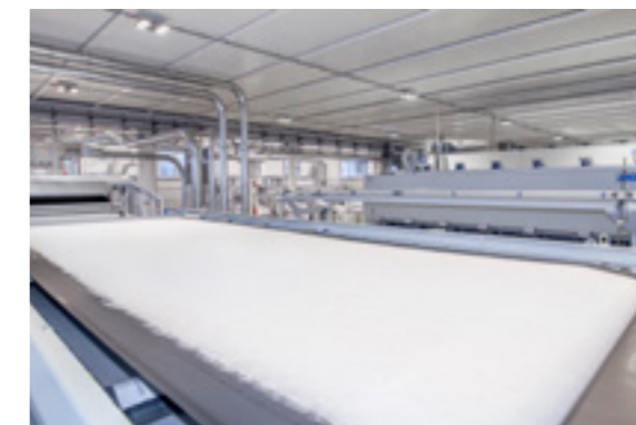
Profile crosslapper with ProDyn and Isolayer systems for improving weight evenness
