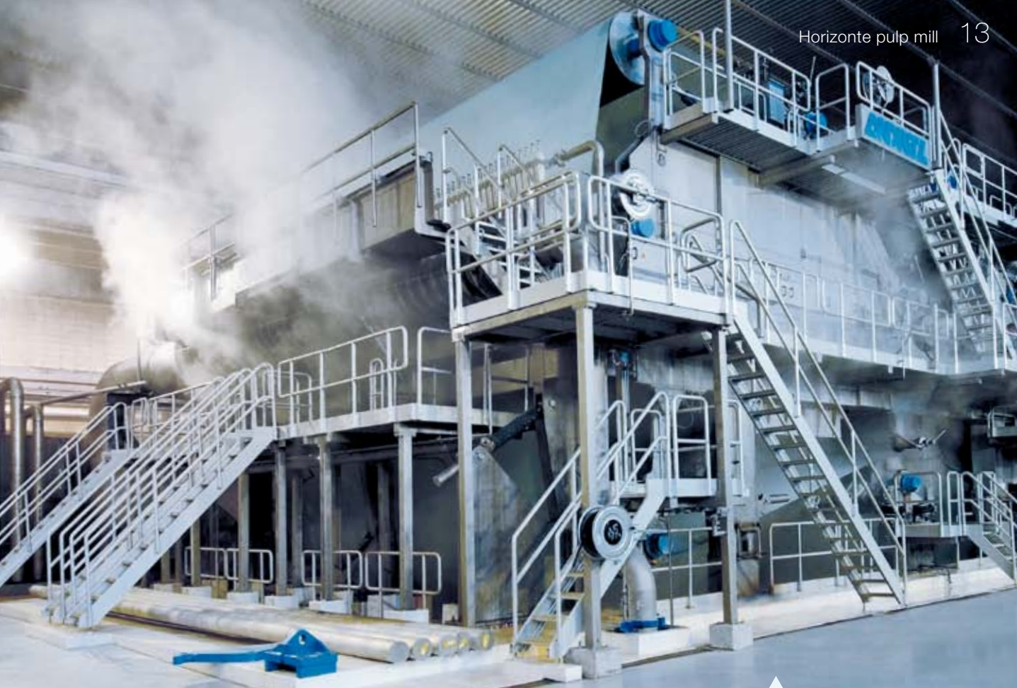
Technology of world-record size: the wet end of the dewatering machine – part of ANDRITZ's scope of supply for Fibria.
