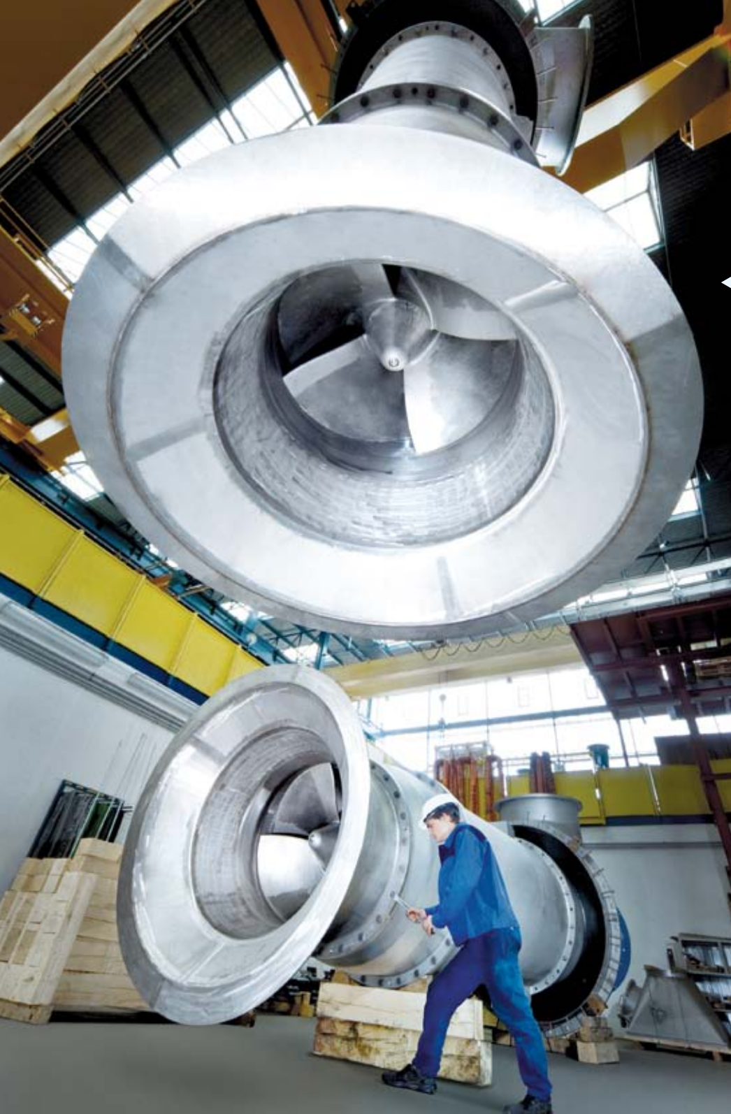
Vertical line shaft pumps made of stainless duplex steel for a power station in Belgium. These cooling water pumps will transport sea water.
